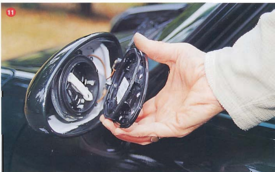
11 Last job is to fit the glass. Push it into place and then use a screwdriver under the lower edge to rotate the locking ring. Now it's time to do the other side!
