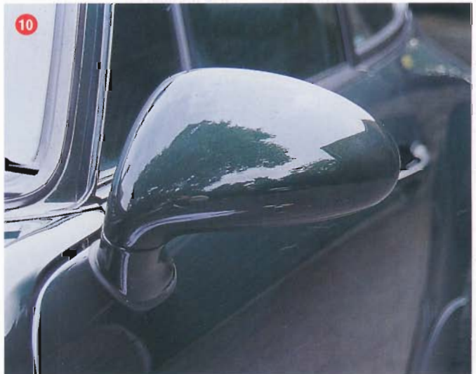
10 Check that the mirror moves in both planes when you operate the adjuster switch. Then bolt it into position, ensuring that the two lugs and the clamp nut locate in their holes
