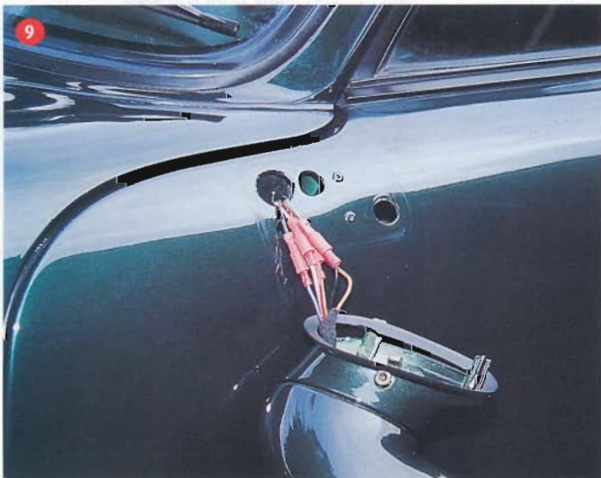
9 Fit the gasket on the base and then push the crimp connectors together, matching the colours as indicated in the panel on page 68. Transfer the bolt and its shaped nut from the old mirror
