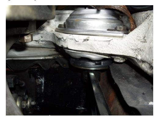
Here are the old mounts. They don't look too bad but when shaken I could hear hydraulic fluid sloshing around which indicates that they had leaked and were therefore were no longer capable of absorbing shocks transmitted from the engine:
