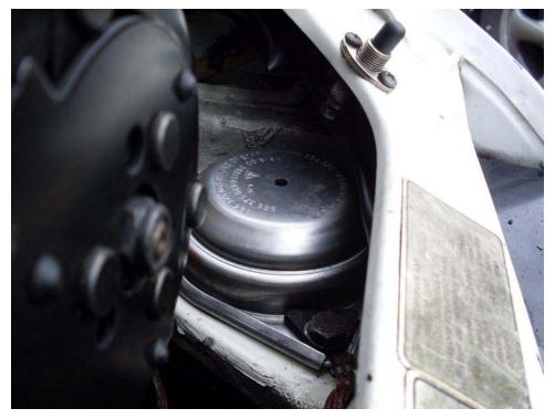
Compared to the old mounts the pictures below show there is only a small gap between the mounts and the frame.
