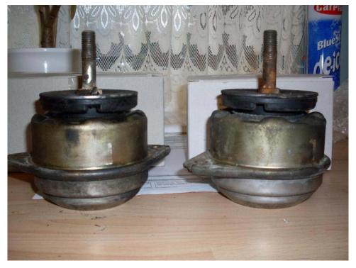
With new mounts gear shifting is much better and the rear of the car settles much quicker when going over bumps.
