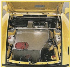
Trunk is stuffed with huge fuel cell. Interior is as luxurious as any you'll find in a pure racing car; second seat is for an instructor.
