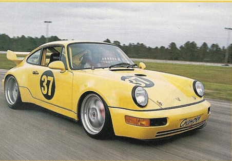
Brakes are lifted from a 911 Turbo S but with racing pads. Porsche says the naturally aspirated flat six produces 320 hp; we say 375.
