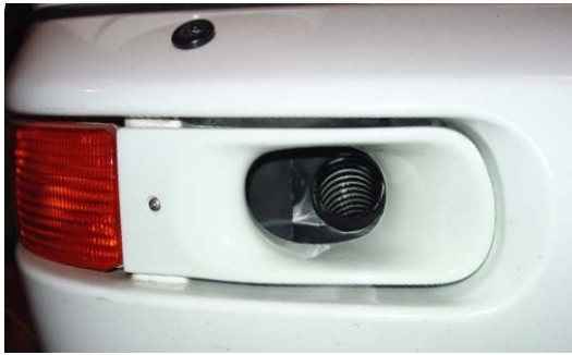
Scoop replaces foglamp to route air to inner fender for additional brake cooling.
