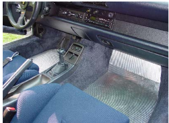
Textured aluminum sheet protects factory foam padding. Floor mats sit on top for daily drive.
