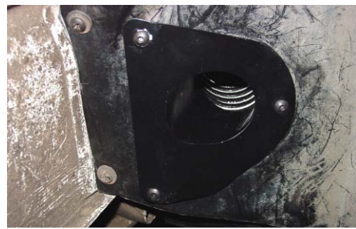
Scoop replaces foglamp to route air to inner fender for additional brake cooling.
